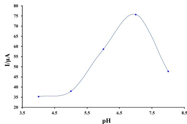
Fig. 4. I-pH curve for electro-oxidation of 500 μM nalbuphine was recorded MgO/CNTs/PI/BMMS/PE.
